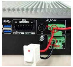
For testing purpose, you can refer to the picture blow to simulate ignition signal input controlled by a latching switch.
